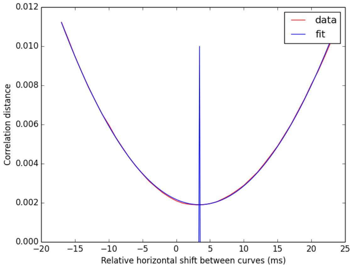
The red curve is the actual data, and the blue curve is a polynomial fit to the red curve, with the actual minima determined from the fit curve to increase precision.
