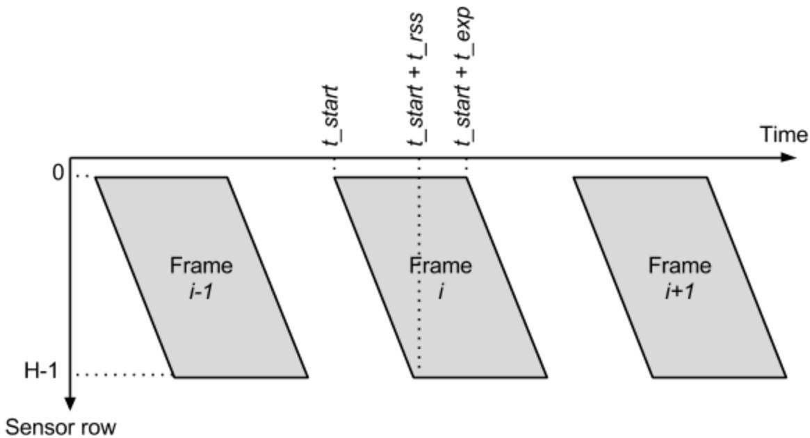
The first step in computing the camera rotation samples is to assign a single time to each frame. This is computed as the “middle” time for that frame, which in the above figure corresponds to a point in the exact center of each parallelogram. The equation for this is:
