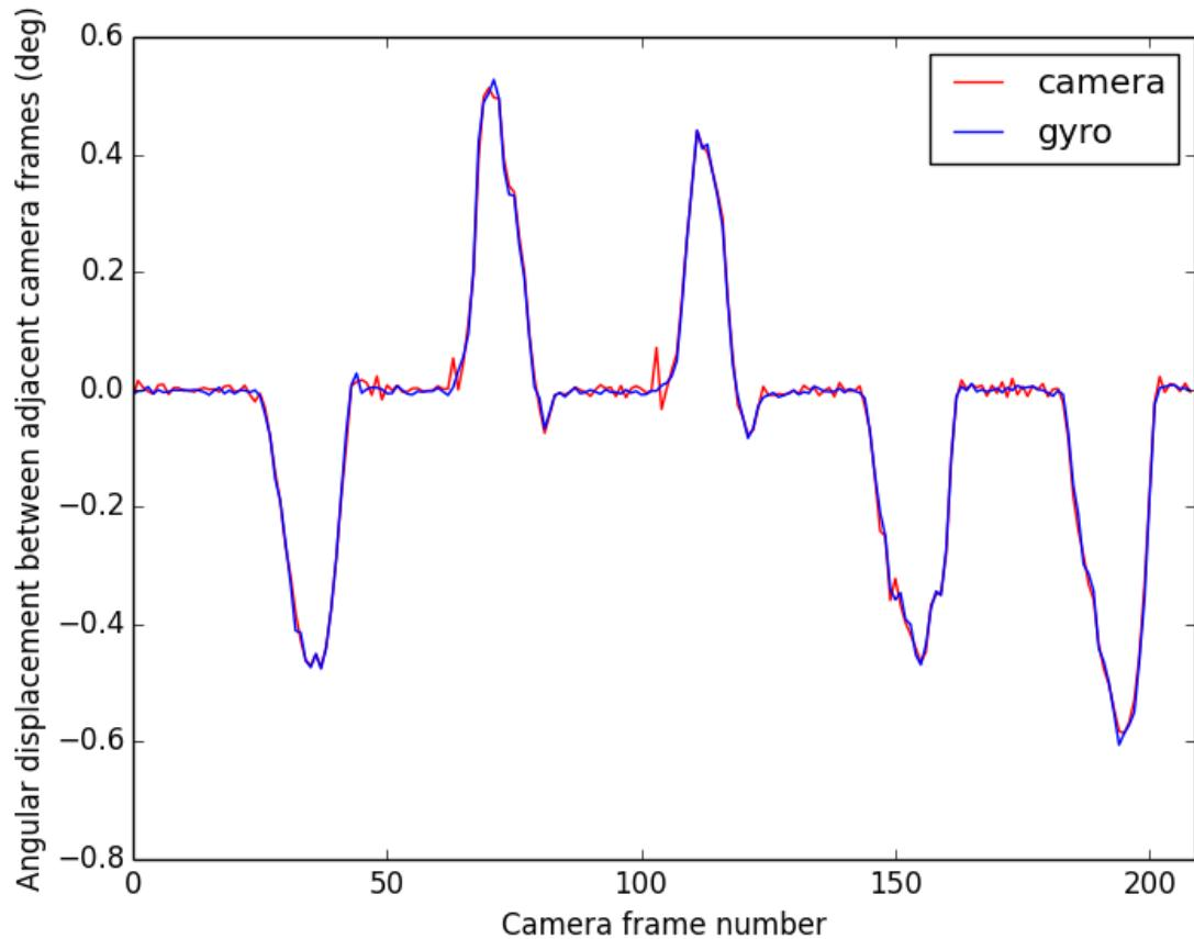
The motions of the user during the test run are evident from this trace; there were alternating periods of 10-20 deg/sec rotation and periods of no motion.
